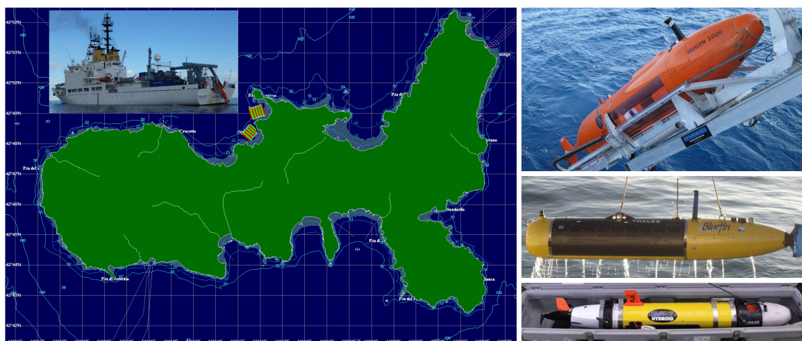
Figure 1: Left: NRV Alliance with the HUGIN-HUS AUV during the MANEX'13 trials overlaid on map of the Italian island Elba highlighting the two common survey areas (green and red stripes in the north of the island). Right: AUV's from top to bottom: HUGIN-HUS, MUSCLE, REMUS100.
